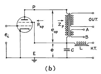
Fig. 1—Series-fed transformer-coupled amplifier (a) triode connection (b) pentode connection.
