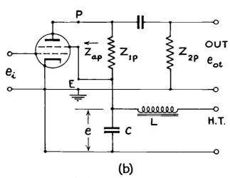
Fig. 2—Parallel-fed amplifier (a) triode connection (b) pentode connection.
